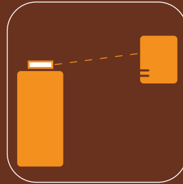
Fig. 5 On a ledge, opposite to the indoor unit
